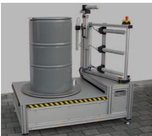
Drum measurement system "light": In 2008, Marschelke Messtechnik developed the DL scanner for dose rate monitoring only on behalf of the Jülich Research Centre
